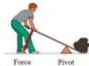
A lever tilts on a pivot which is nearer to the end of the pivot with a heavy load.
